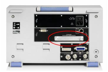
This removes all user data from the oscilloscope. The oscilloscope, **without** the removable hard drive, can now leave the secured area. Once the oscilloscope is outside the secured area, installing a second **non-classified** removable hard drive (without any user data), allows the digital oscilloscope to function properly for service or other needs.
